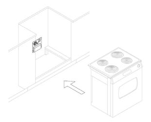
Thanks to the special slim design of SPO-32 in which overall projection from the wall surface (pavement) does not exceed 22mm. This small projection of the device makes life easy when installed behind the electric range, 30cm above floor level and never interfere with the electrical range back-side and or decoration.
