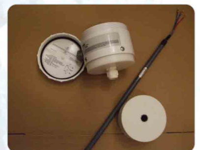
AWAM main parts, Connection Head, Probe Tube and Float Cylinder.
